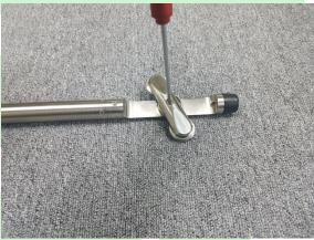
② Unscrew the star wrench bolt, wheel yoke and torsion spring by using a T25 star wrench.
