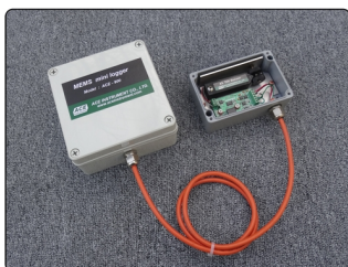
[MEMS inclinometer connection]
