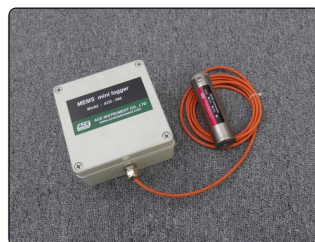
[ELS inclinometer connection]
