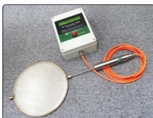
[Measurement of earth pressure]
